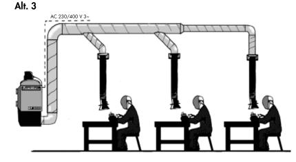
Central system: 3 X LM-2 connected to one electrostatic filter EF type. Recommended filter per no. of arms: EF-2000: 1-2 arms\* EF-3000: 1-3 arms\* EF-5000: 2-5 arms\* When more stations are required the system can be fitted with ASE-12 automatic dampers.
