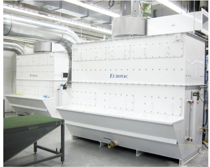
*Type "A" Central Wet Collectors - Sludge Rake Dust Removal*
